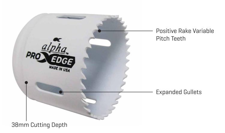
Alpha PROEDGE Bi-Metal holesaws are fast and clean cutting multi-use holesaws. They are suitable for drilling wood, nail embedded wood, plastic, stainless steel alloys and mild steel.
